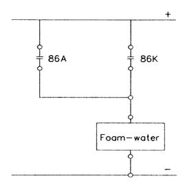
17.14 Signals of indoor fire protection system of each room and signals of outdoor fire protection system of each transformer shall be sent to local CCS, GCC, RCC, and NCC as following details;
